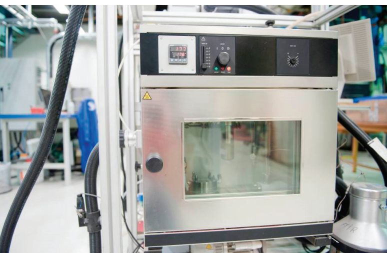
Figure 21: FTIR gas sampling and conditioning unit. Photo: Sascha Njaa, SINTEF
